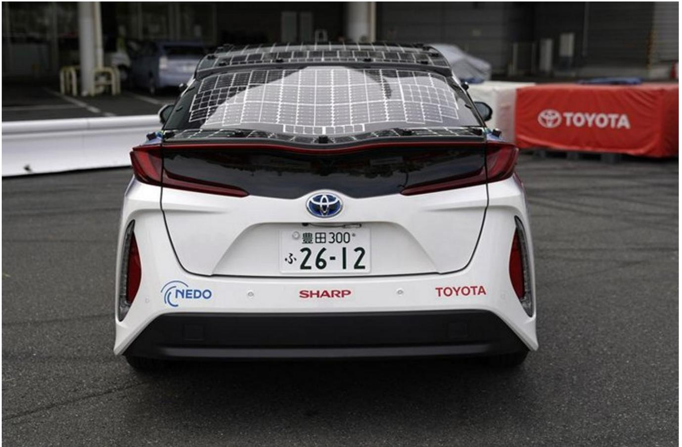
Toyota is working on a solar-powered car that could essentially keep on going without needing any sort of external charging. The project is a work in progress by Toyota Motor Corp. in collaboration with Sharp Corp., and the New Energy and Industrial Technology Development Organization of Japan(NEDO).
